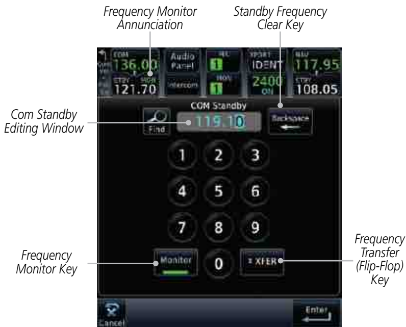
Figure 3-19 Com Frequency Monitoring
