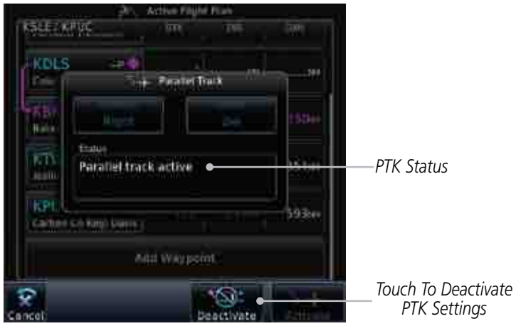
Figure 4-30 Deactivating Parallel Track
